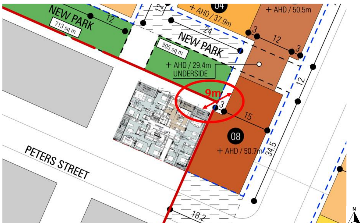
Figure 38: Envelope plan - height of building in storeys plan showing NW-2 block and relationship to adjoining approved development to the southwest at 8-12 Peters Street (level five floor plan)
