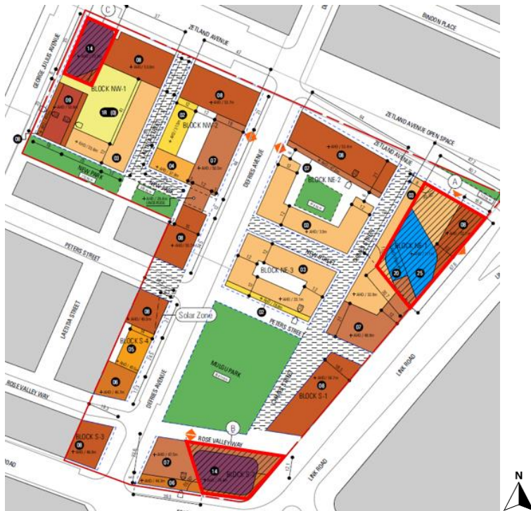
Figure 45: Building Envelope Plan showing location of tower zones hatched and outlined in red
