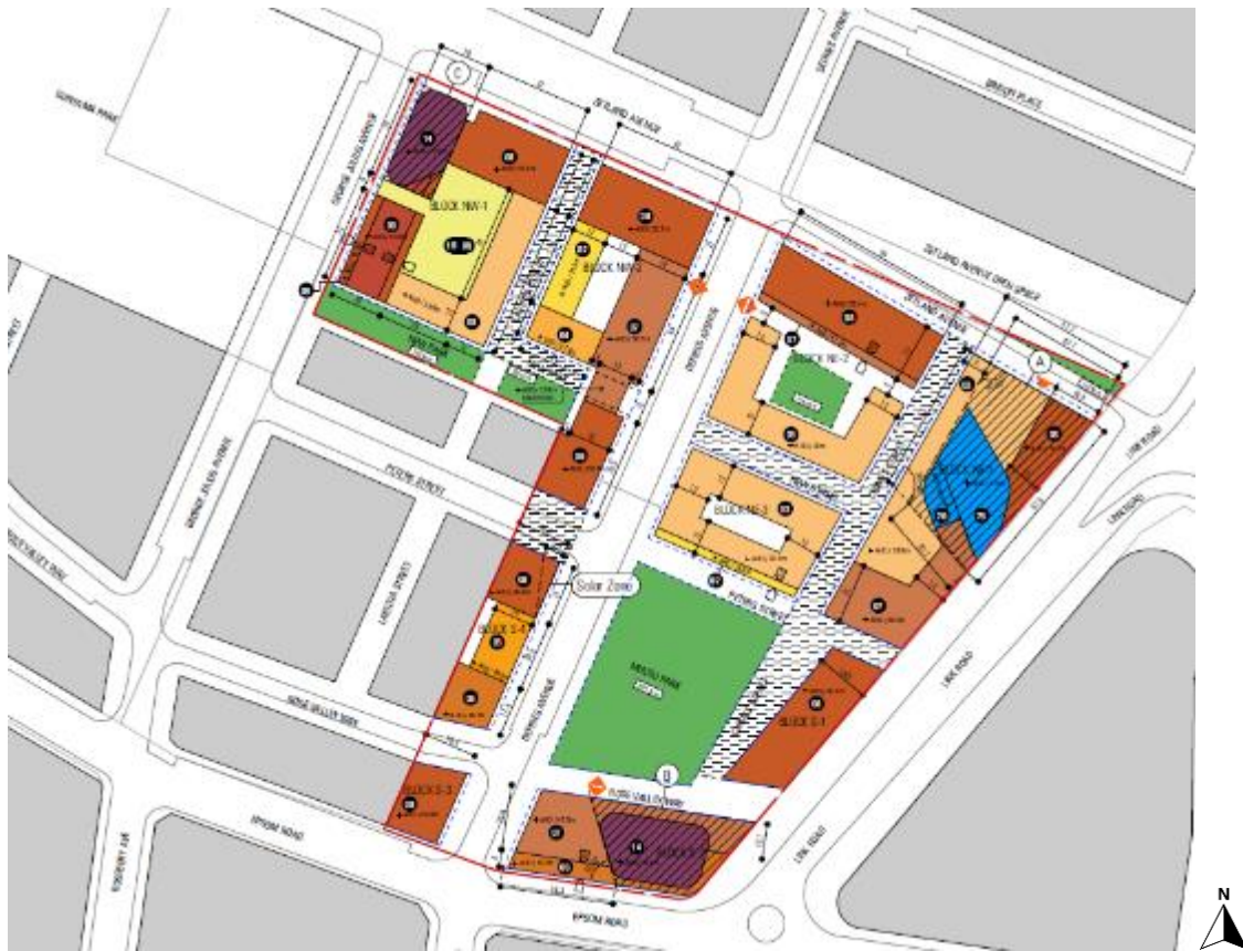
Figure 15: Envelope Plan - height of storeys
