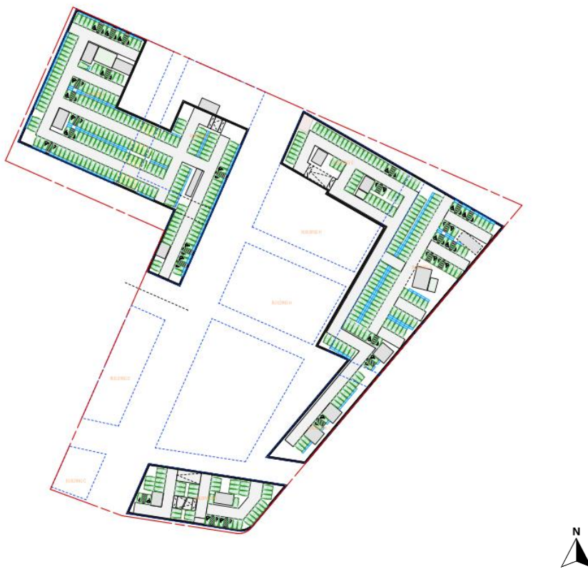
Figure 18: Reference Scheme - level two basement plan
